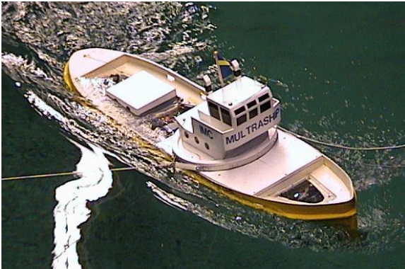
Fig. 1 Scale model of the carousel on a conventional Combi tug
