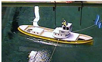
Fig. 12 Capsize testing with sideward snap loading
