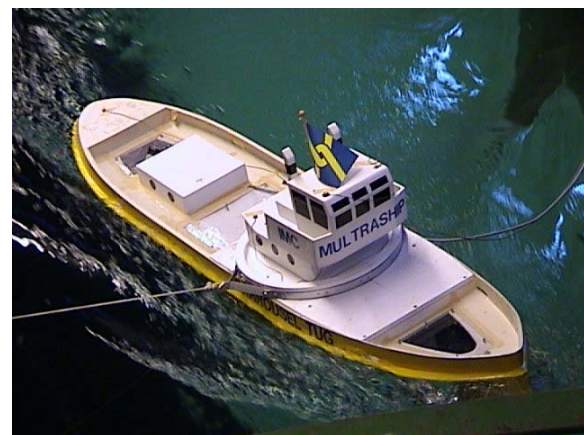
Fig. 10 Sailing ahead / wire over side (~ 60 ton)
