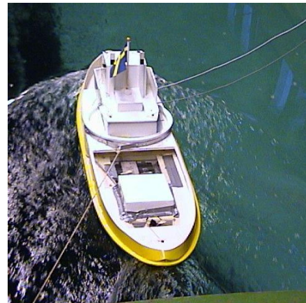
Fig. 9 Sailing ahead / wire over stern
